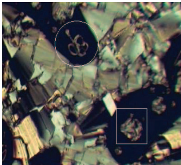
Figure 3. Photomicrograph showing the 'free-moving' filament (in circle) which coalesces to form the broken focal-conic texture (in square) of compound 6 at 174.4°C during the second heating.
